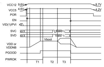
Figure 4. SVI-Mode Power-sequencing Diagram
