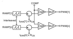
Figure 9. Circuit Channel Current Balance
