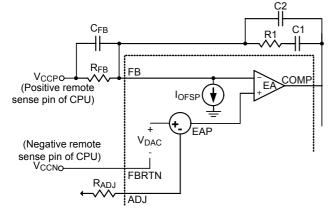
Figure 7. Circuit for VCORE Differential Sensing and No Load Offest
