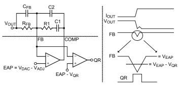
Figure 8. Load Transient Quick Response
