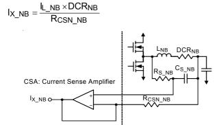
Figure 12. Current Sensing Circuit for NB Section
