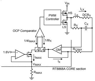
Figure 11. Over Current Protection for CORE Section
