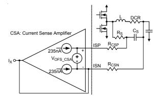
Figure 5. Current Sensing Circuit
