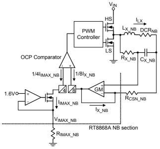
Figure 13. Over Current Protection for NB Section
