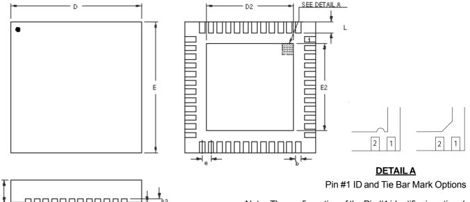
Note : The configuration of the Pin #1 identifier is optional, but must be located within the zone indicated.
